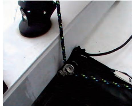
4:3 Take the free end of the halyard through this cleat; it is underneath the spinnaker chute, and it may need to be moved for the pulley to be exposed.
