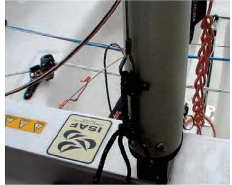
3:5 Tie the jib sheets onto the eye on the clew of the jib.
