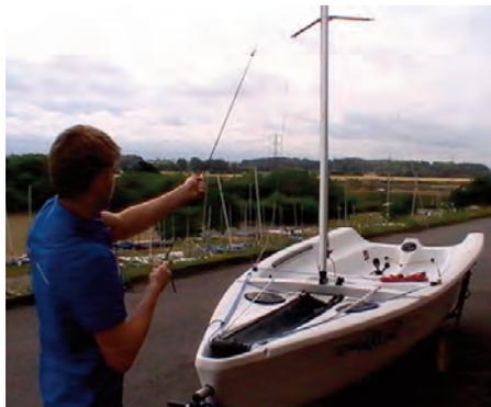
1:7 Having pulled the mast upright, secure the forestay around the black furling bar. Ensure all halyards are clear and not twisted.
