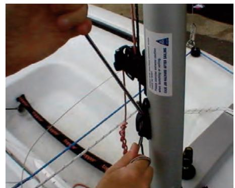
3:4 Once the rig tension has been applied, the forestay can be moved back from the bar at the front and then tied off to the mast.
