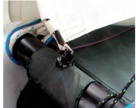
TIP: Wrap some electrical tape around the furler. This will protect the spinnaker from the sharp split ring and help to prevent rips in the sail.
