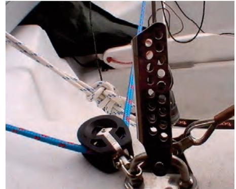
1:5 Fix the base of the mast to the mast step on the cross beam with the pin and ring from the mast step.
