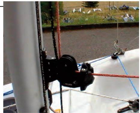
2:4 Now thread the mainsheet. Starting from the centre cleat on the hull (NB: ensure the the ratchet clicks when the rope is pulled in), go up to the rear block, and thread the line back to front. Then go to the pulley on the two thin lines, and thread it back to front. Then go to the front pulley on the boom, and thread it front to back. Finally, the main sheet goes to the pulley on the strop and through the hole in the centre of the pulley. Tie a stopper knot to prevent the line unthreading.
