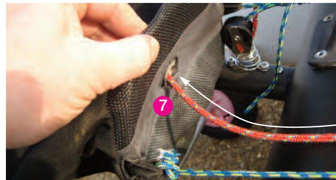
H. (8) Feed end of spinnaker halyard through the spinnaker chute until the tail comes out the front of the chute. (Tip; it is easier to do this by fishing the spinnaker halyard out of the chute with a tiler arm or similar long object in order to feed it from the back of the chute to the front).
