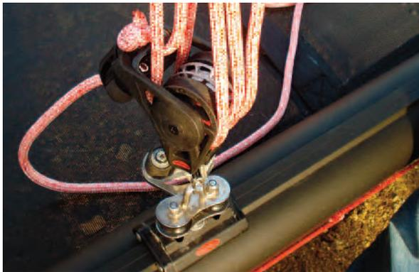
B. Feed tail end through cleat on carriage and then through double pulley block.
