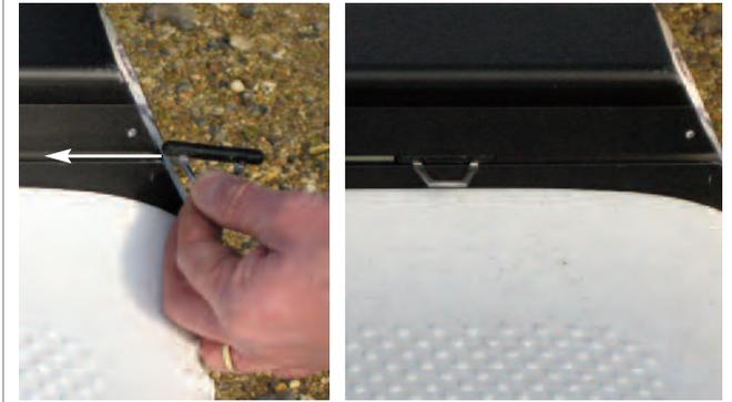
E. Re-affix beam end caps to secure trampoline in position.
