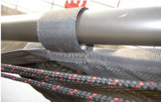
C. Then attach back of spinnaker sock around either side of the base of the mast.
