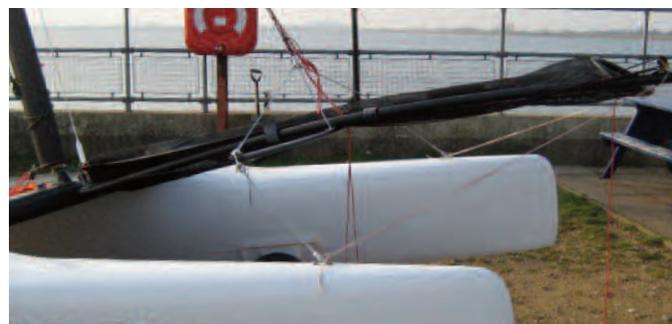
E. (1) Take line from the chute mouth and (2) tie off on to the eye on the front of the hull.
