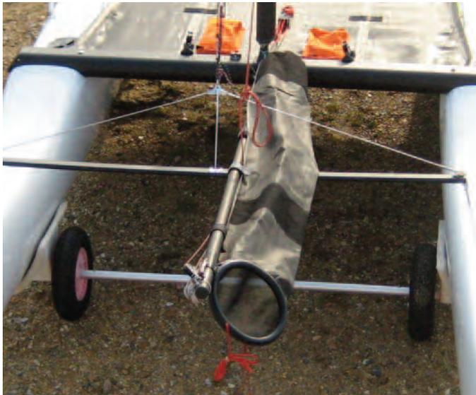
Attach velcro straps around spinnaker pole.
