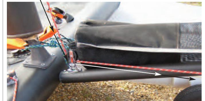
Remove the rope that is securing the double block to the spinnaker pole (this is for shipping purposes only).
