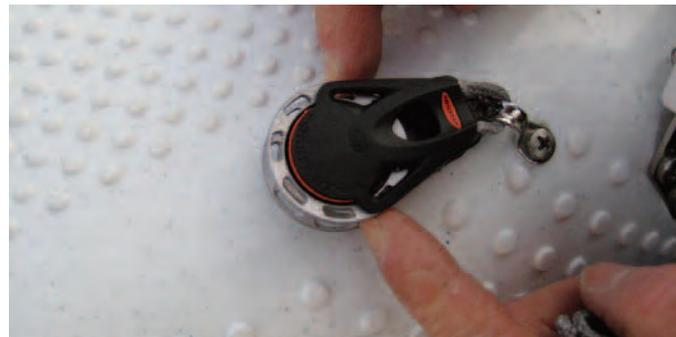
Feed spinnaker sheets through ratchet blocks and attach to the Clew of the spinnaker sail.
